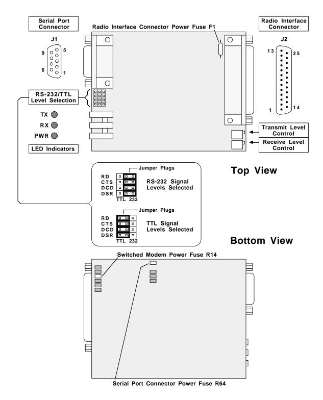
Fuse F1 is a through-hole 1 amp picofuse, fuses R14 and R64 are 1 amp 1206 surface mount fuses.
