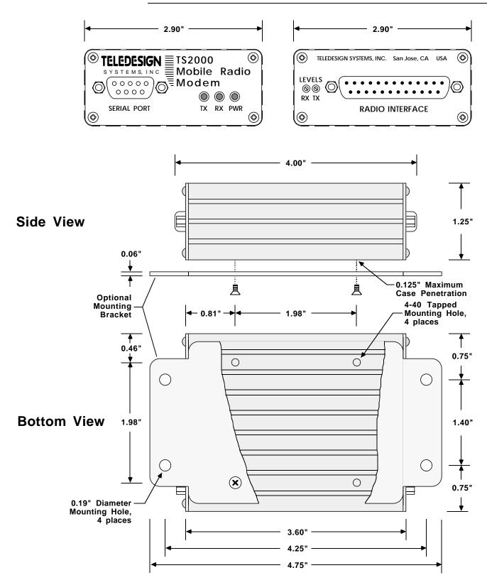
The mounting bracket may be rotated 90 degrees to support an optional mounting position with the 0.19" mounting holes positioned on each side of the TS2000 case instead of at the front and rear.
